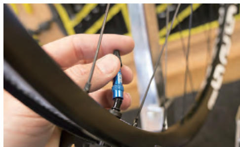
INSTALL VALVE STEM
